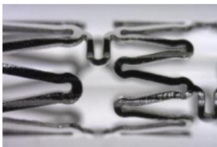
Figure 5. Optical microscope image of EP treated SUS stent cut by fs-laser.
